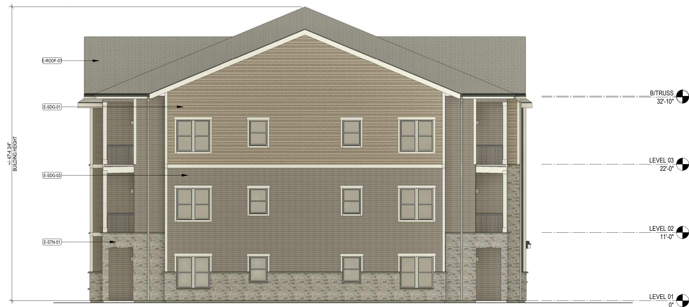
4 Elevation- Exterior- Side- Large Bldg - Color 1/8" = 1'-0"
