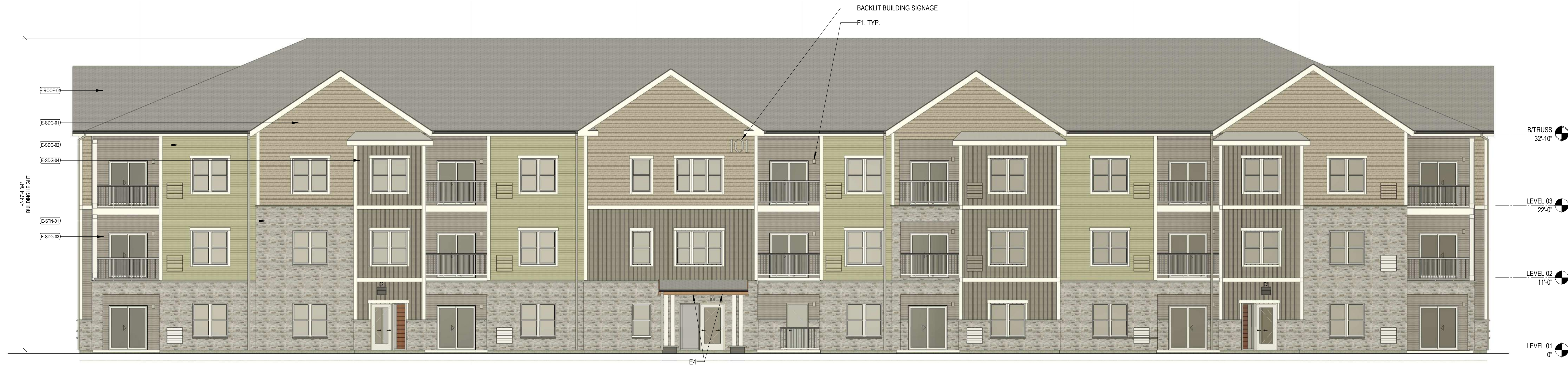
2 Elevation- Exterior- Front- Bldg Type A & F 1/8" = 1'-0"
