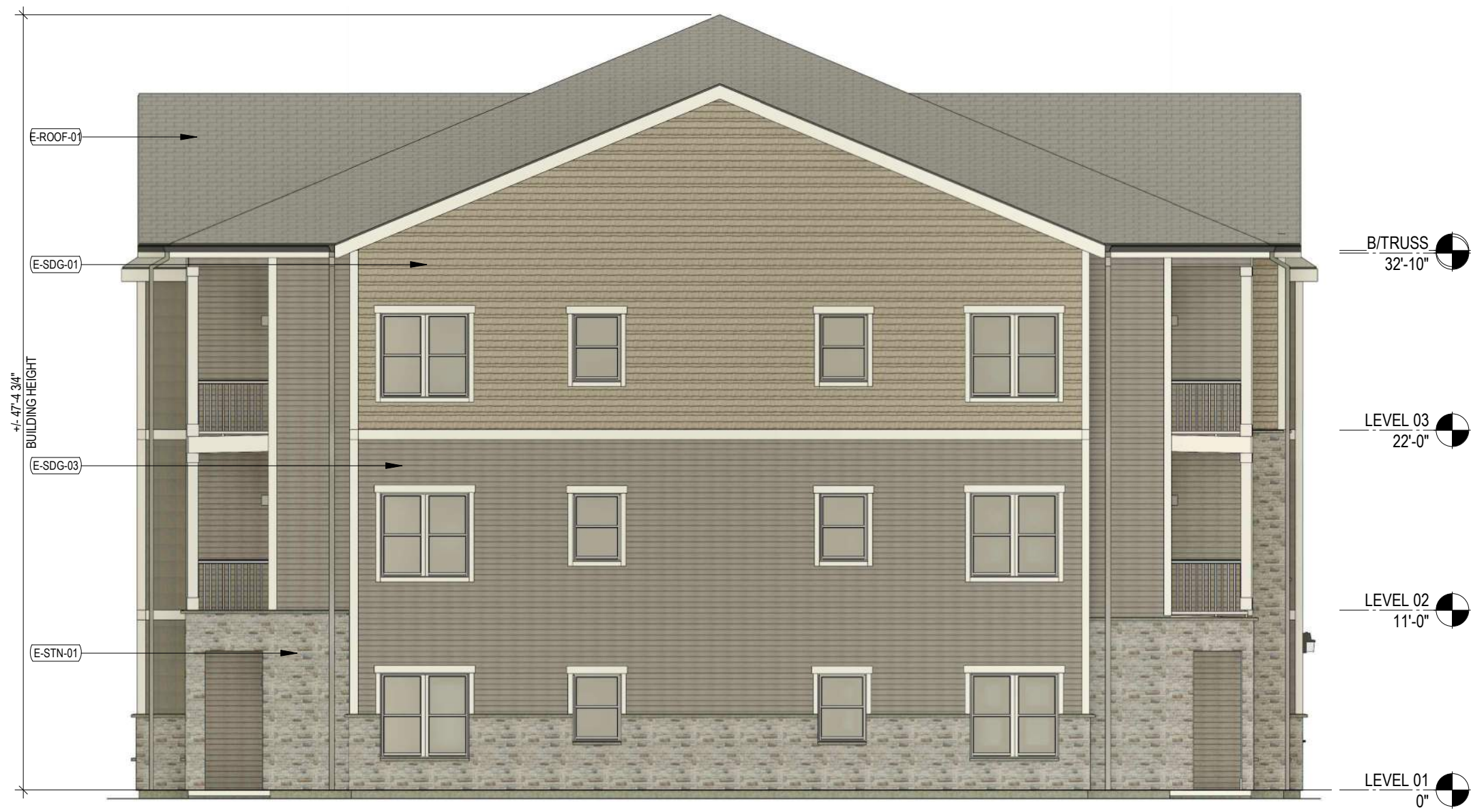
3 Elevation- Exterior- Side 2 - Bldg Type A & F 1/8" = 1'-0"
