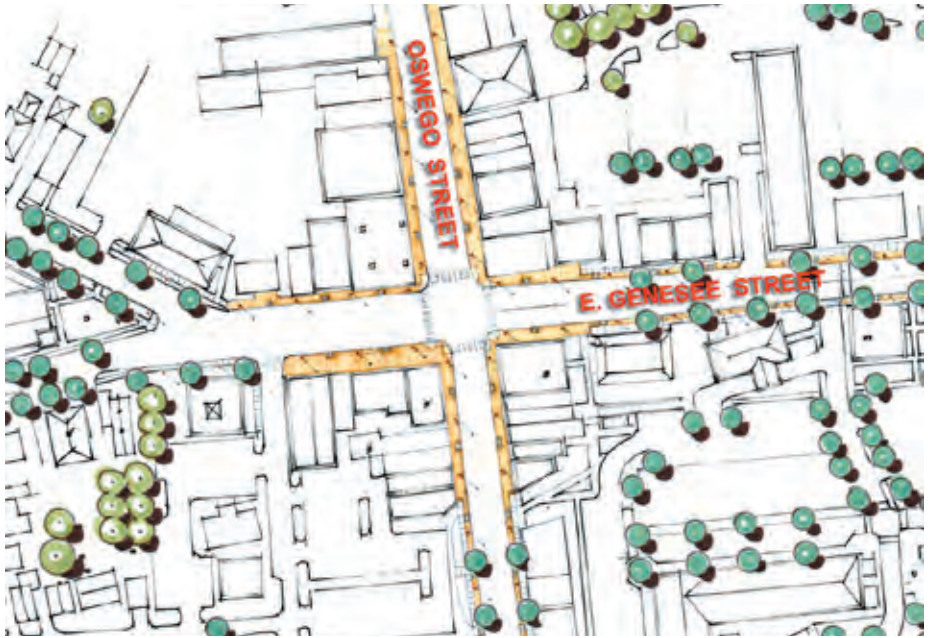
Recommended sidewalk treatment plan for the Four Corner area
